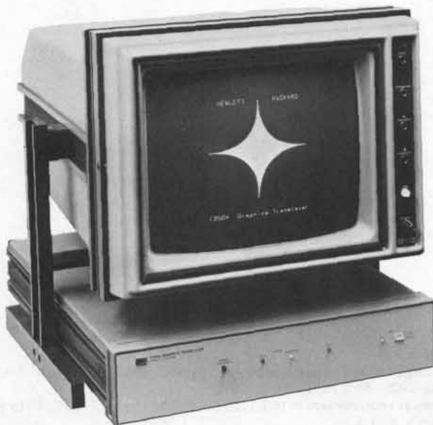
The 1350S Display System includes a 1311 X-Y Display, a 1350A Graphics Translator, an interconnecting cable, and a binder for instruction manuals.
