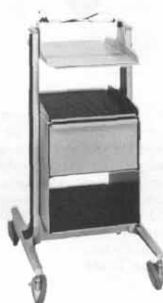
Opt 005: storage cabinet and drawer in upper position with shelf on top; load limit 18 kg (40 lb) ea on shelf and in cabinet, 11 kg (25 lb) in drawer.
